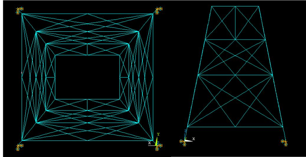
Cross section of the antenna is square beams assembly
